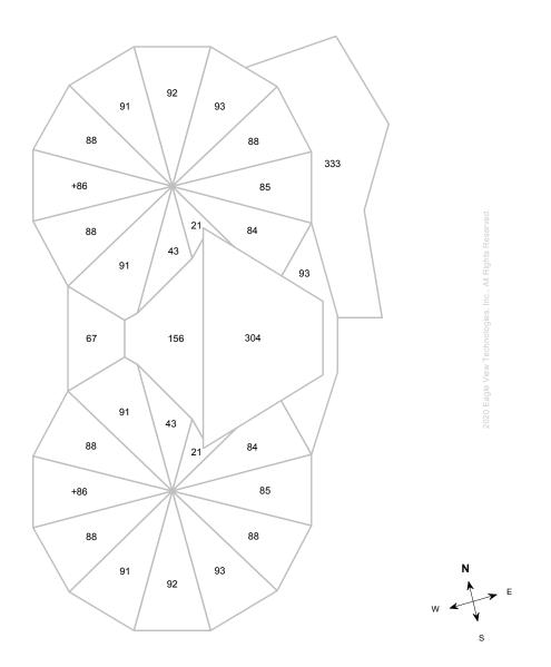
Note: This diagram shows the square feet of each roof facet (rounded to the nearest Foot). The total area in square feet, at the top of this page, is based on the non-rounded values of each roof facet (rounded to the nearest square foot after being totaled).
