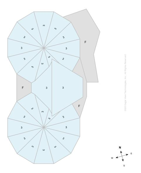
Note: This diagram contains labeled pitches for facet areas larger than 20.0 square feet. In some cases, pitch labels have been removed for readability. Blue shading indicates a pitch of 3/12 and greater. Gray shading indicates flat, 1/12 or 2/12 pitches. If present, a value of "F" indicates a flat facet (no pitch).
